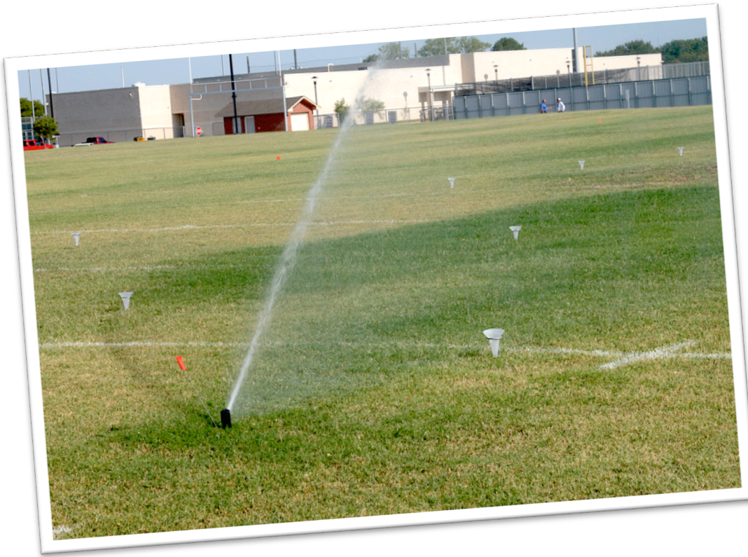
Figure 3: Conduct irrigation audit to make sure irrigation system is working as efficiently as possible. Darker green bermudagrass was due to irrigation head not rotating.
